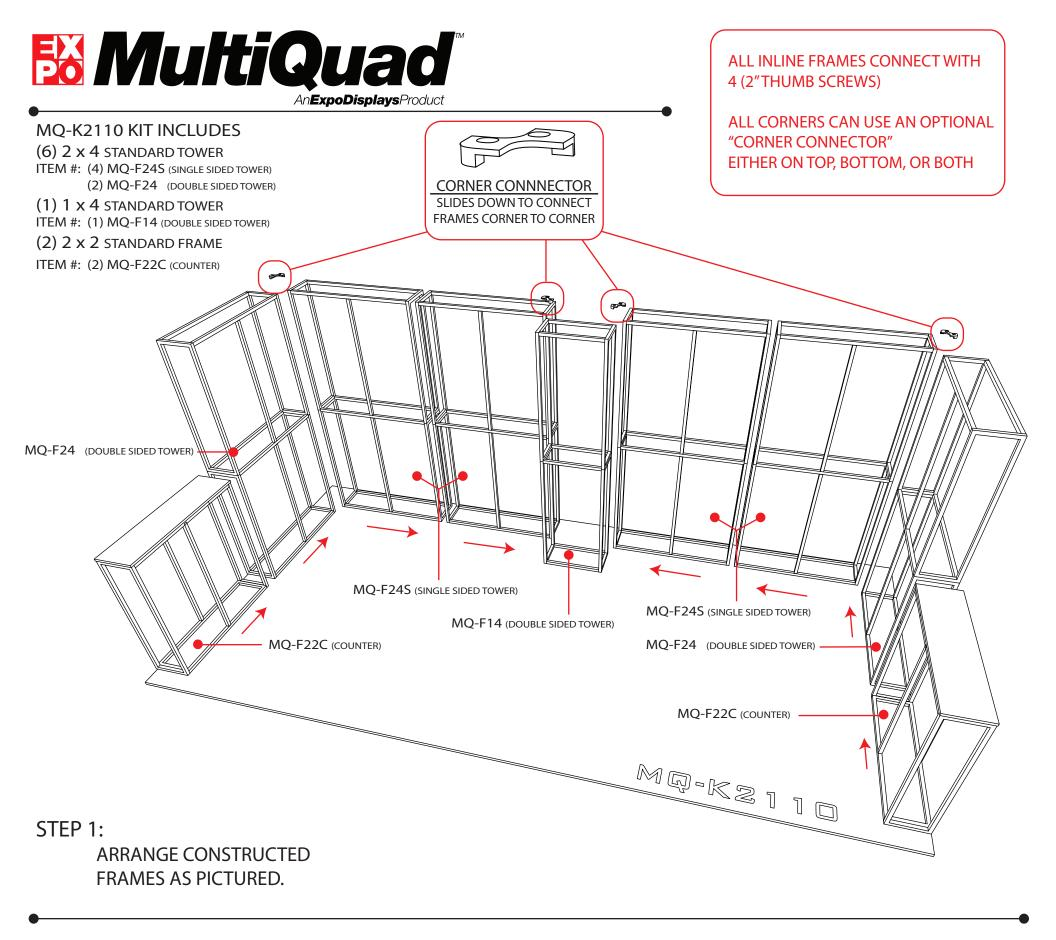
STEP 2: SECURE FRAMES WITH 2"THUMB SCREWS AND CORNER CONNECTORS (IF NEEDED).
